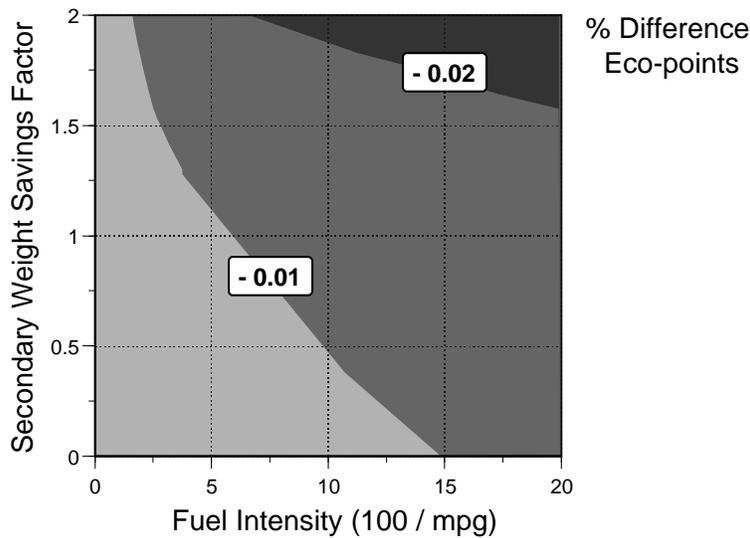
Figure 7. Relationship between secondary weight savings, fuel intensity, and percent difference in eco-points (Eco-Indicator 99)
