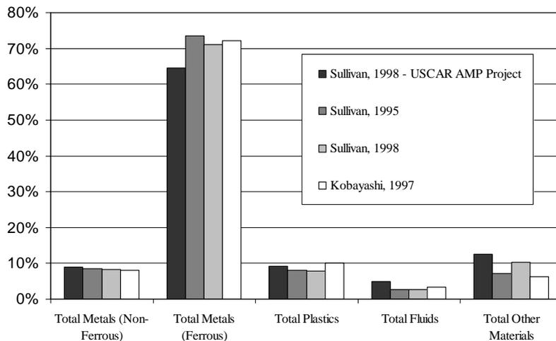
Figure 2. Comparison between material compositions used in vehicle LCA studies
