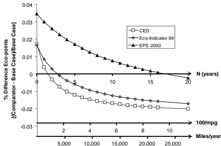
Figure 5. Comparison of Comparator and Base Case vehicles using Eco-Indicator, EPS, and CED varied across intensity of use (i.e. measured in terms of vehicle life, fuel consumption, and miles/year) – includes production, use, maintenance, and end-of-life
