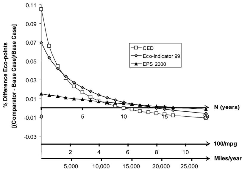
Figure 6. Comparison of Comparator and Base Case vehicles using Eco-Indicator, EPS, and CED varied across intensity of use (i.e. measured in terms of vehicle life, fuel consumption, and miles/year) – includes production, use, and maintenance (excludes end-of-life)
