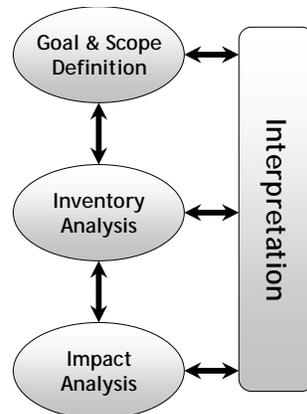
Figure 1. ISO 14040 framework for LCA [7]
