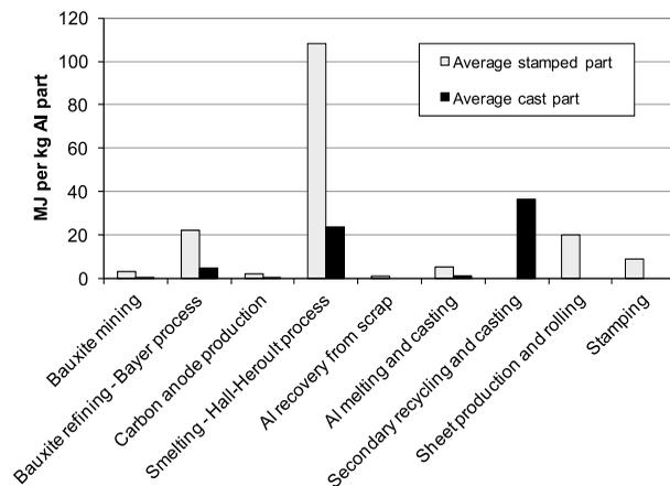
**Figure 5** Production energy requirements for automotive aluminum parts in 2000, by processing stage.
