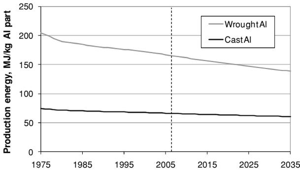
**Figure 6** Production energy requirements for automotive aluminum parts over time.
