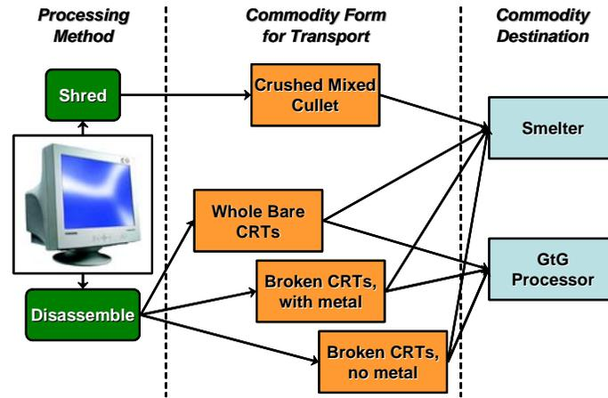
**Figure 2. Recycling alternatives for CRT glass from Monitors/TVs for a first tier processor.**
