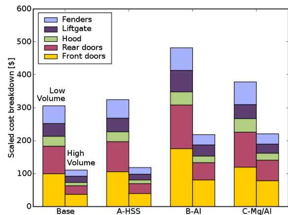
Figure 4 Scaled cost breakdown by subsystem of representative closure set at annual production volumes of 20,000 / yr (first bar) and 150,000 / yr (second bar)
