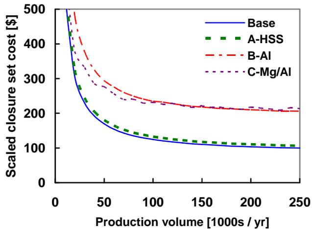
Figure 1 Scaled unit cost of representative closure set as a function of production volume
