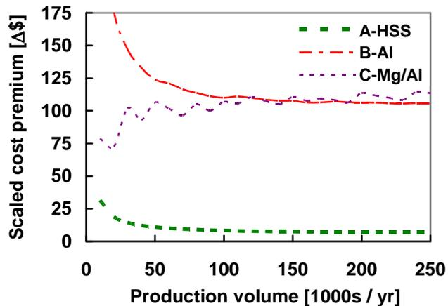
Figure 2 Scaled unit cost premium over mild steel (MS) of representative closure set as a function of production volume
