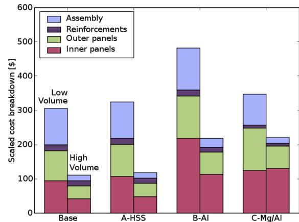
Figure 3 Scaled cost breakdown by part and assembly of a representative closure set at annual production volumes of 20,000 / yr (first bar) and 150,000 / yr (second bar)
