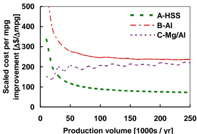
Figure 7 Scaled cost per MPG improvement ( $\Delta\$ / \Delta\text{mpg}$ ) as a function of production volume for representative designs
