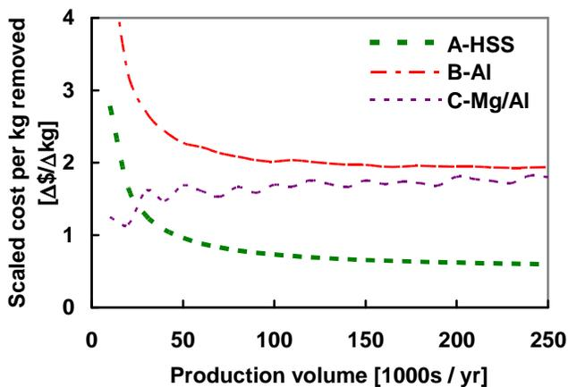
Figure 6 Scaled cost per kilogram removed ( $\Delta\$ / \Delta\text{kg}$ ) as a function of production volume for representative designs
