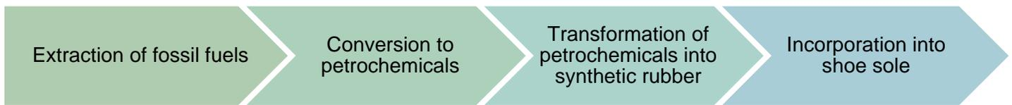
Figure 1 Steps in the processing of synthetic rubber for footwear (International Institute of Synthetic Rubber Producers Inc.)
