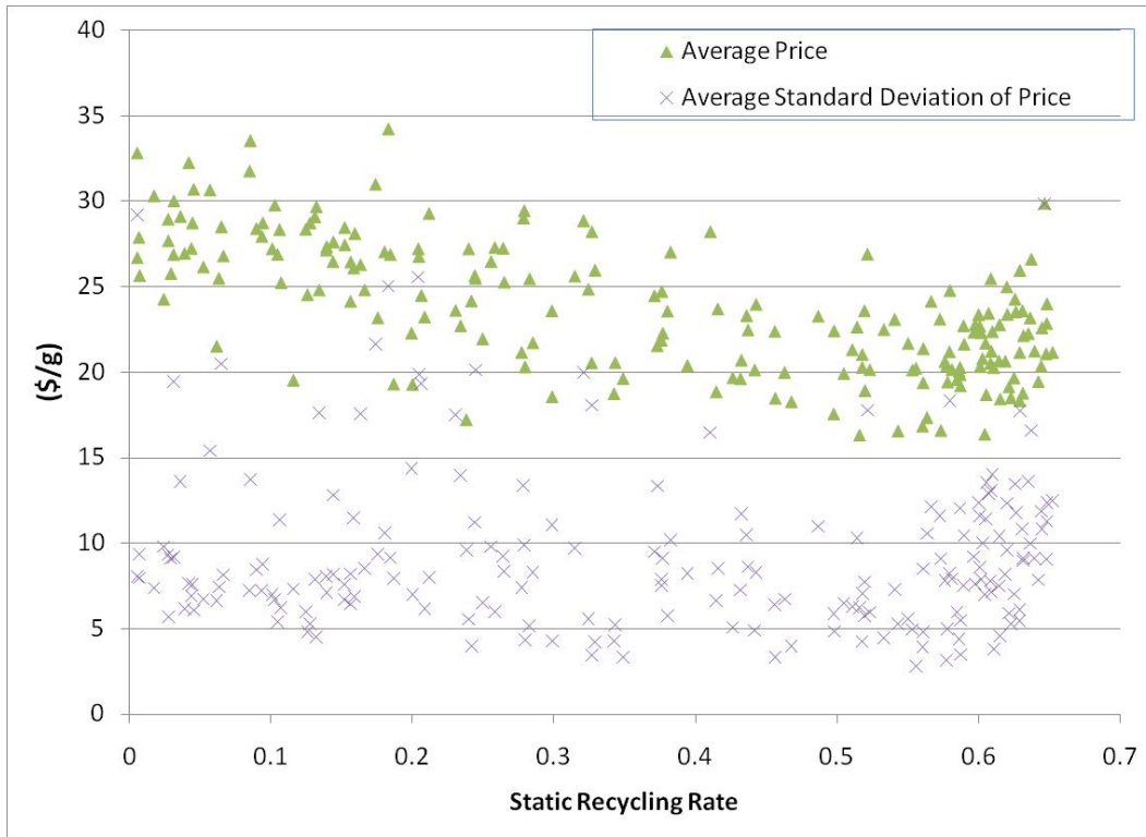
Figure 55: Zero-growth Scenarios. Average price and average standard deviation of price are plotted for each simulation run at varying recovery rate multipliers selected randomly for the sensitivity test. The results from 200 simulations are plotted as a function of measured average recycling rate.
