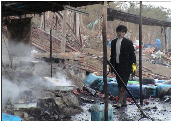
Laborer heating aqua regia acid mixture along riverside chemical stripping operation to extract gold from imported computer chips. All waste acids and sludges are dumped into the river. The only protective equipment used are rubber boots and gloves. © BAN
