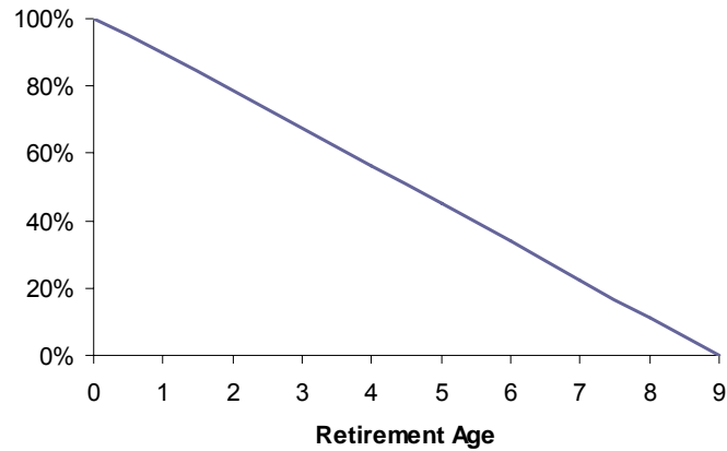
Figure 8: It is estimated that the probability that a one-year-old product is still functional is 0.90.
