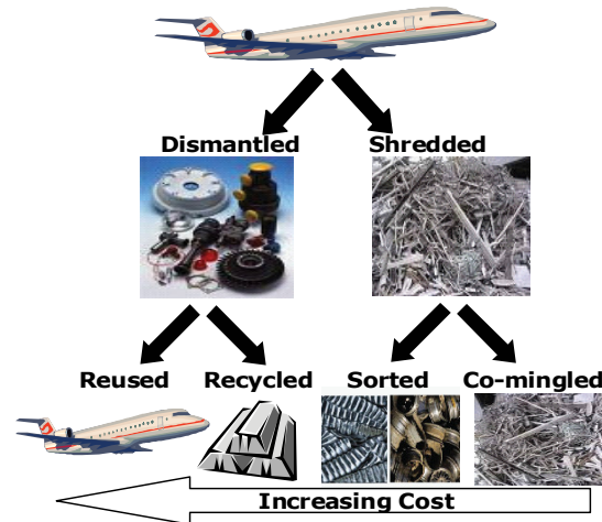
Figure 33. Schematic of various end-of-life recycling and/or reuse options for aerospace scrap
