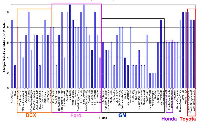
Figure 15: Sub-Assembly Operations Performed Inside OEM Plants<sup>26</sup>
