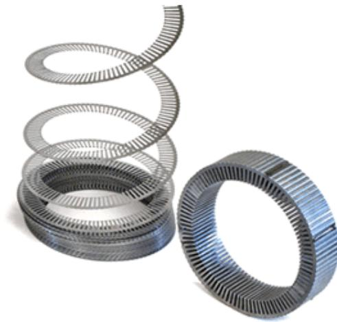
Figure 64: Example of how a stator core is manufactured using the "Slinky" method. Photo courtesy Precision Pressing Manufacturers (36).
