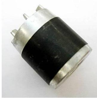
Figure 2: Finished induction rotor core with aluminum as the conducting material. Photo courtesy Bühler Group (11).
