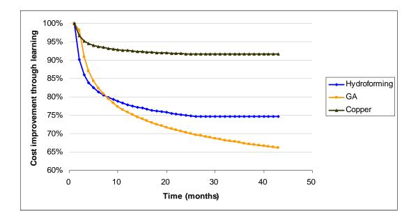
Figure 44: Cost learning curves for tube hydroforming, car general assembly, and copper wire
