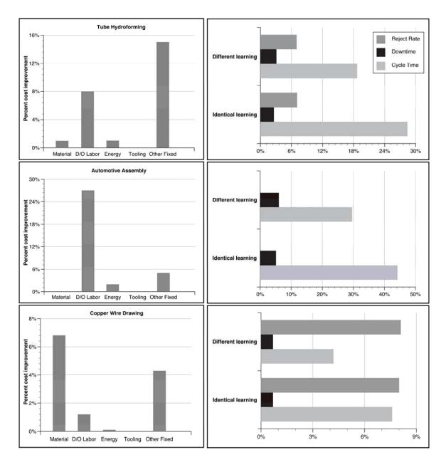
Figure 43: Left - Percent of initial cost saved through learning by cost element for (a) hydroforming;(b) general assembly; and (c) copper wire drawing processes. Right - Cost improvement by operational parameter, for identical and differing learning rates and scopes.
