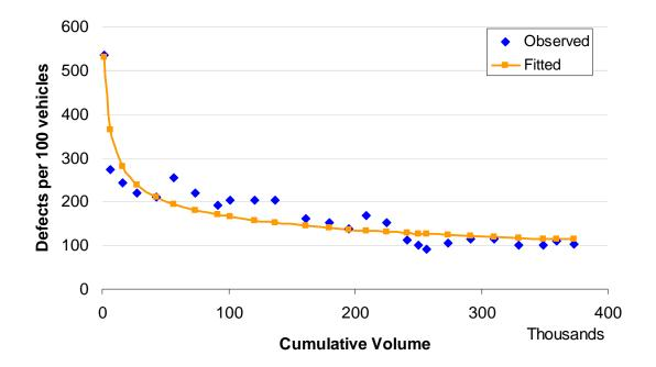
Figure 10: Log linear regression of defect rate data vs. cumulative volume
