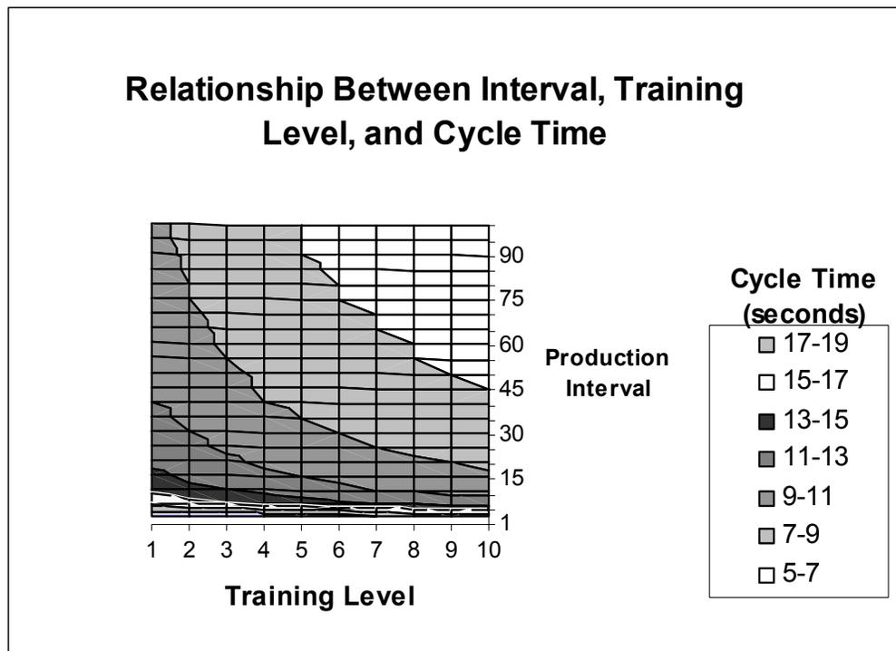
Figure 8: Relationship Between Production Interval, Training Level, and Cycle Time
