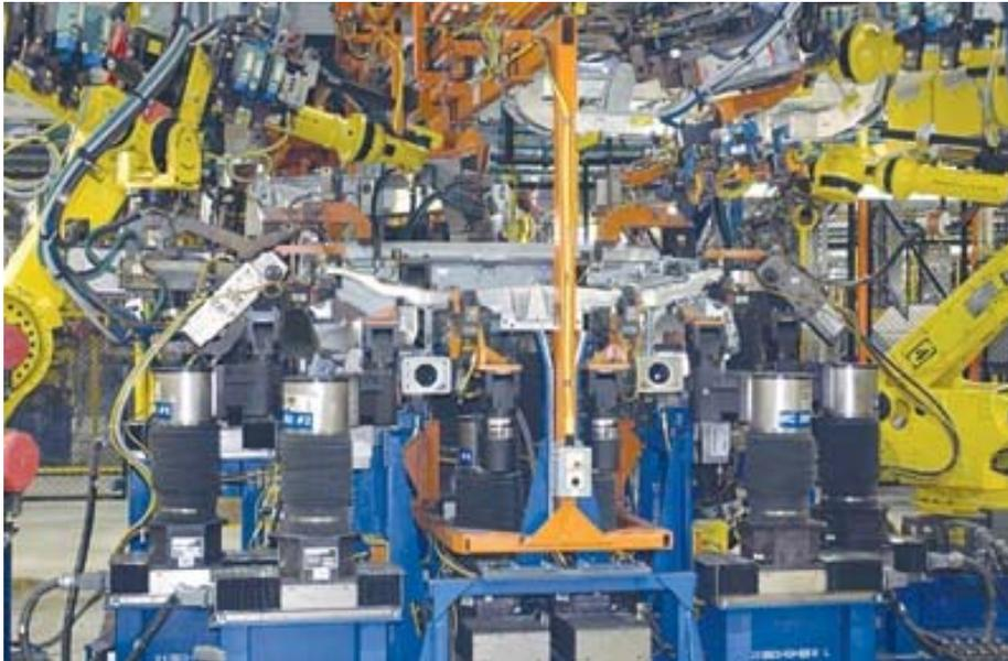
**Figure 2.1:** Station comprised of several PRRT units surrounded by RSW robots. The PRRTs are the smaller piston type arms<sup>21</sup>.
