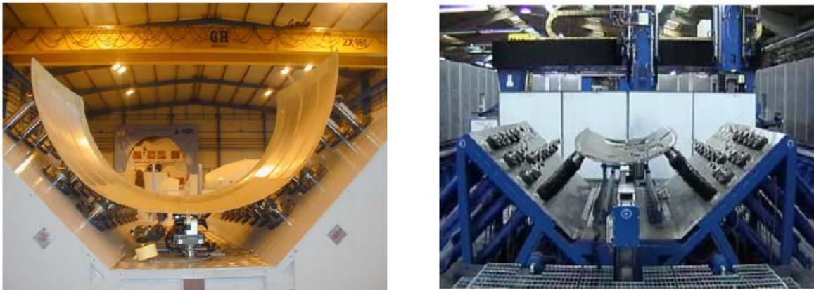
**Figure 5.1:** Bombardier Aerospace technology: **a)** tricept tooling and **b)** axis nacelle tooling<sup>3</sup>.
