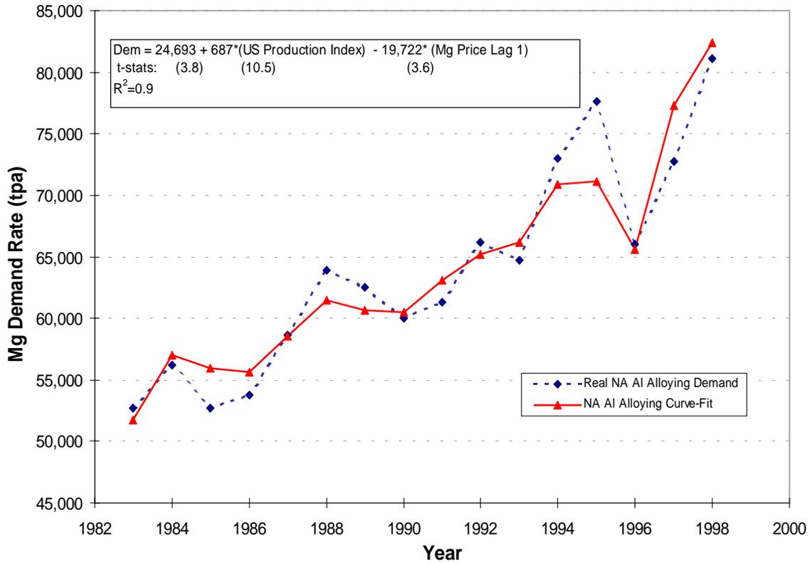
**Figure A-3: North American Aluminum Alloying Mg Demand and Econometric Curve-Fit**
