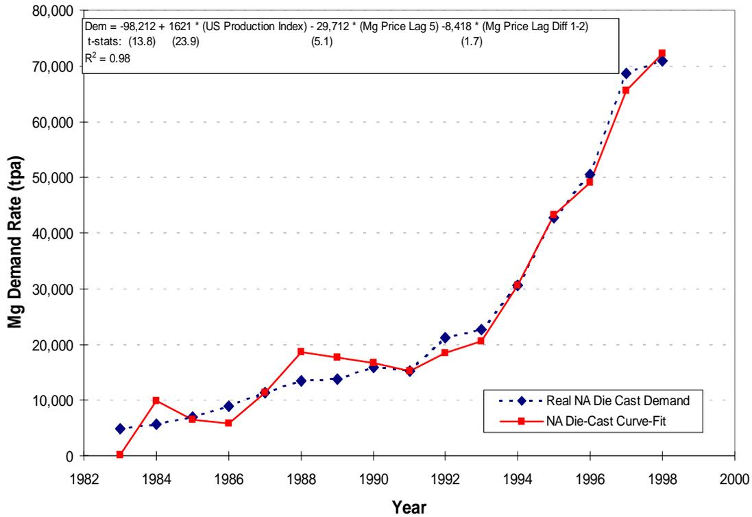
Figure A-1: North American Die-Cast Mg Demand and Econometric Curve-Fit
