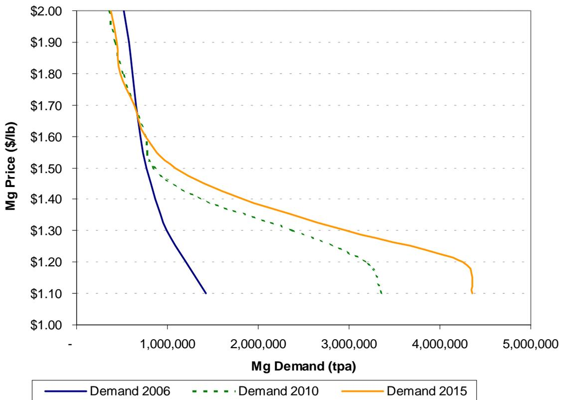
**Figure 26: Yearly Total World Magnesium Consumption Potential Under Long-term Constant Material Pricing**
