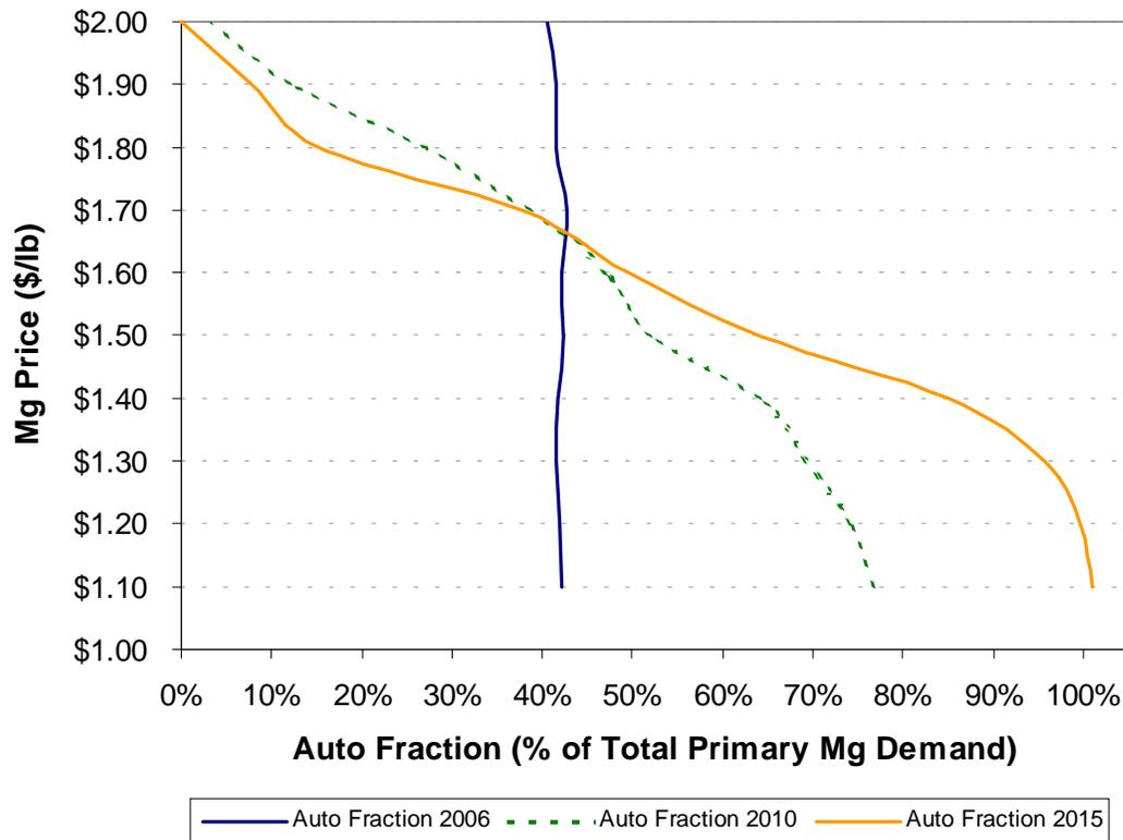
**Figure 28: Automotive Share of Magnesium Consumption Under Long-term Constant Material Pricing**
