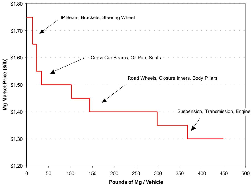
**Figure 6: Magnesium Automotive Design Deployment Price Sensitivity, e.g. North American Large Car**
