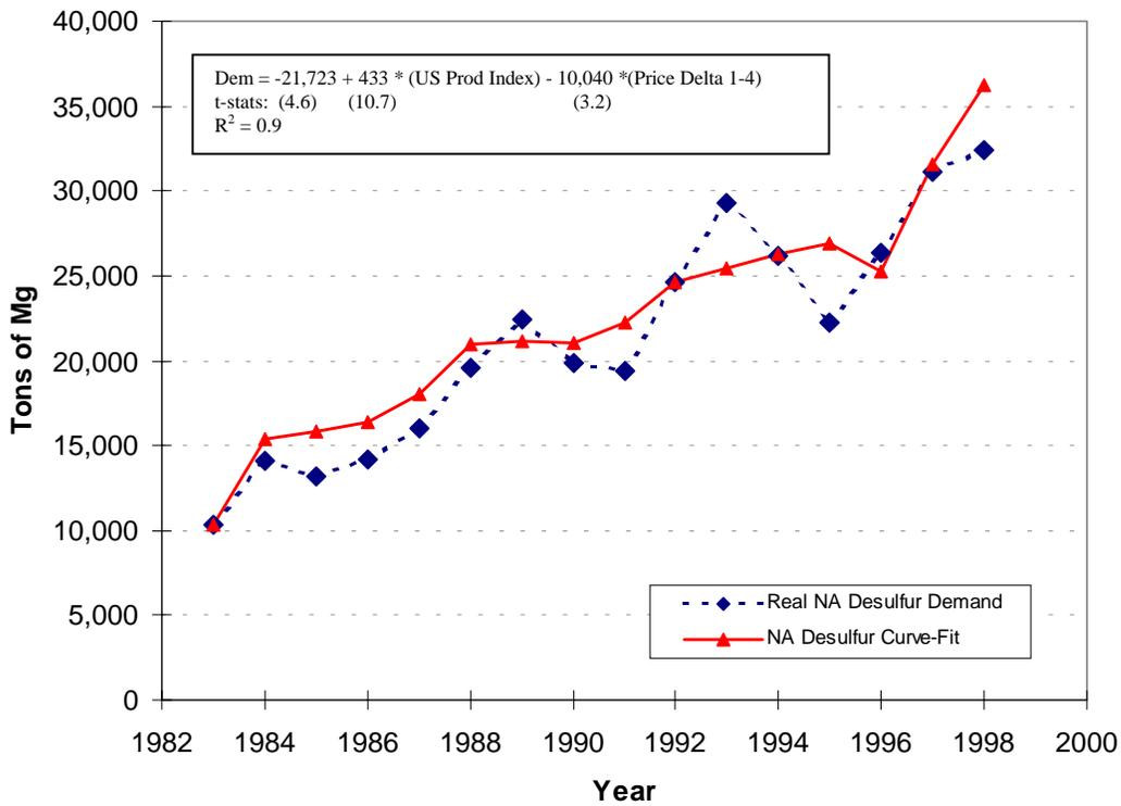
**Figure 14: North American Steel Desulfurization Demand and Econometric Curve-Fit**
