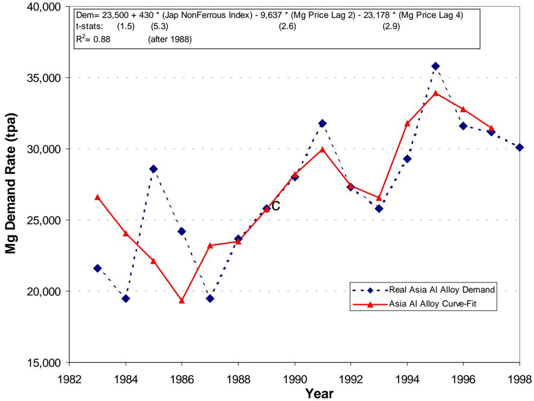
Figure A-11: Asian Aluminum Alloying Mg Demand and Econometric Curve-Fit
